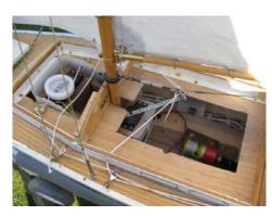
**Folkboat: Sailing Yacht:** (Unfinished project, needs additions and a little modification to running gear). Length 39", Beam 10", Draft 9". Fitted auxiliary motor (500 type), Genoa rig, winch for sails. Receiver and servos, no transmitter. Interesting popular design and sail plan.
