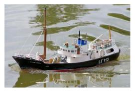
"Boston Arrow" - Fishing Trawler: Length: 37", Beam 8". Tin-Plate/Ply/Plastic Hull. Single Screw, ESC, 40MHz receiver, servos, 9.7V NiCad battery. Rebuilt model with detailed deck fittings.
