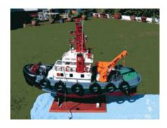
"Toiler IV" - Harbour Tug: Length 22", Moulded Plastics constructon. Single Screw / Vorth Schneider system.
