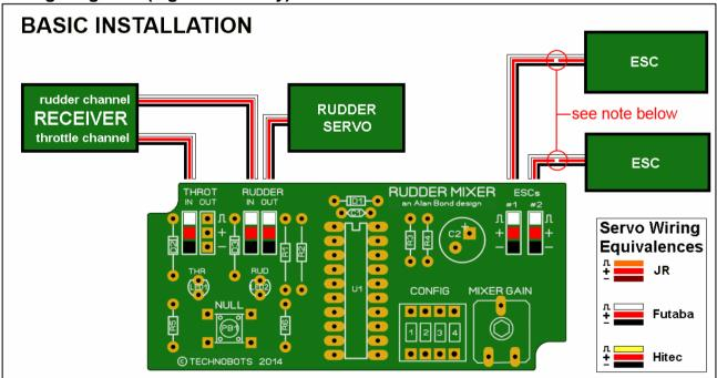
**Note:** if both ESCs have an integral BEC (battery elimination circuit) then one of the BECs should be disabled by removing its red wire from its plug – otherwise the BECs will "fight" each other. If supplying the receiver's 5v supply from a separate battery box and either or both of the ESCs contain integral BECs then the BECs should be disabled. There must be only ONE 5v supply in the installation.
